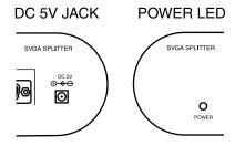
After connecting all cables, turn on the power to your SVGA display before powering your SVGA source.
